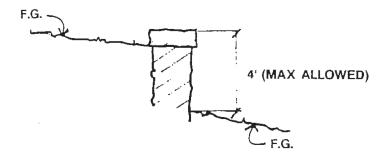
Where slopes require more than 4' of retention, a series of stair stepped walls with planting spaces between will be required
