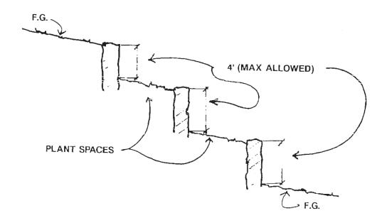
**Allowable Materials:** Stacked Stone, Laid Stone, Timber (with permission of NCC) Stuccoed Concrete with Stone or Brick Cap, Brick or man-made stone (with permission of NCC)
