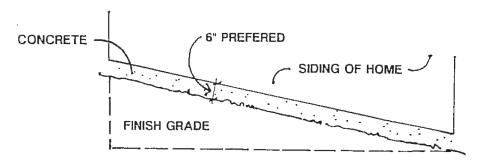
The NCC will allow a maximum of 2' exposure of concrete
